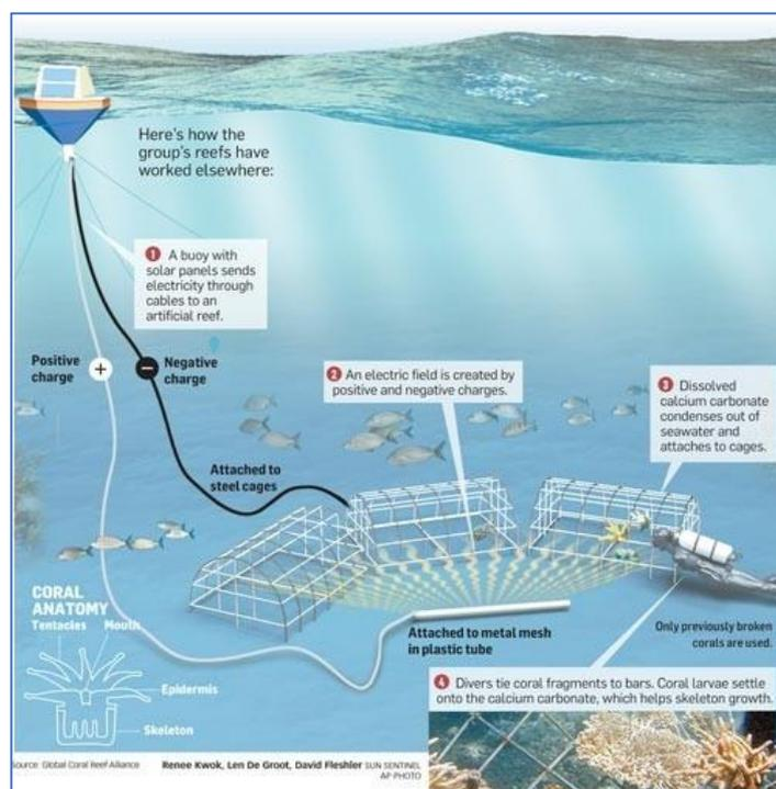
Figure 3 - Overview of Electrolytic Reef Restoration Set Up<sup>29</sup>
