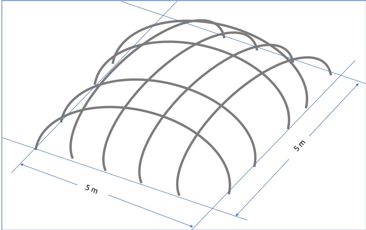
Figure 8 - Schematic of cathode - 5m x 5m rebar domed structure
