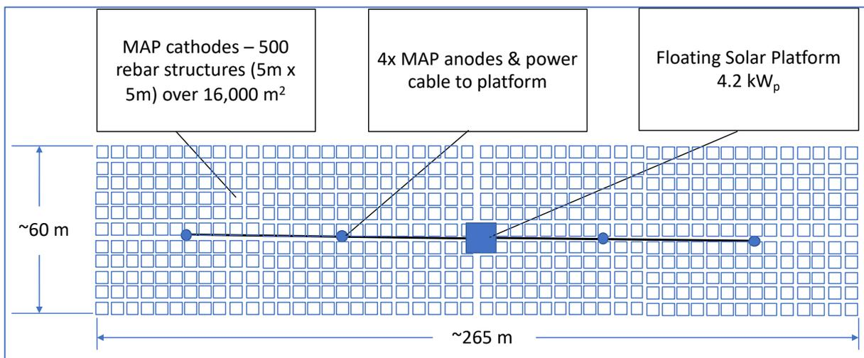
Figure 7 - Conceptual lay-out of 125 rebar domed cathodes - 1 rectangle configuration
